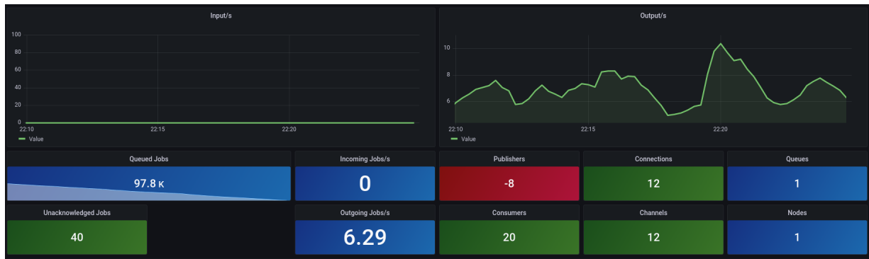
Key metrics on RabbitMQ premade board. Input/s is jobs being published per second. Output/s is the jobs being completed per second, this indicates the total throughput of the system in terms of jobs
